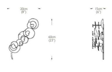
dimensions:  $20 \text{cm w} \times 15 \text{cm d} \times 60 \text{cm h} (8'' \text{w} \times 6'' \text{d} \times 23'' \text{h})$ light source:  $5 \times \text{LED} \text{ total, each } 1 \text{W}, 2700 \text{K, approx } 80 \text{ lumens}$
