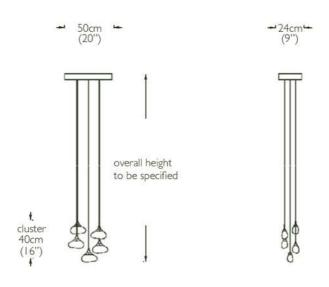
dimensions: oval canopy size -  $50 \text{cm w} \times 24 \text{cm d} (20" \text{w} \times 9" \text{d})$
